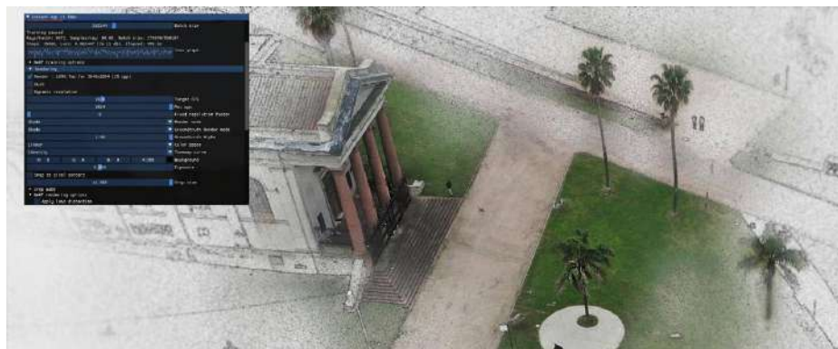
Figure 2. Volumetry generación using NeRF. Source: author's photo
